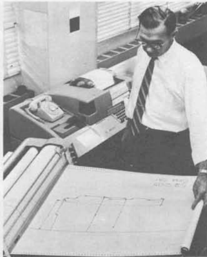
2. Studying printout of Calcomp plotter, George Anderson, manager of engineering, observes tool path for NC lathe. He can thus verify the computer program that creates the NC tape via time-sharing service.
